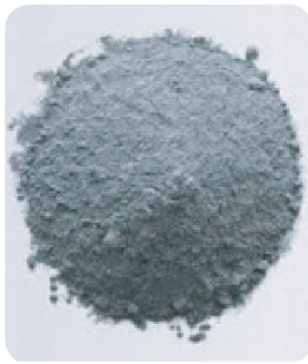
Figure 4: Fine fly ash present in flue gas feed to a carbon capture process
