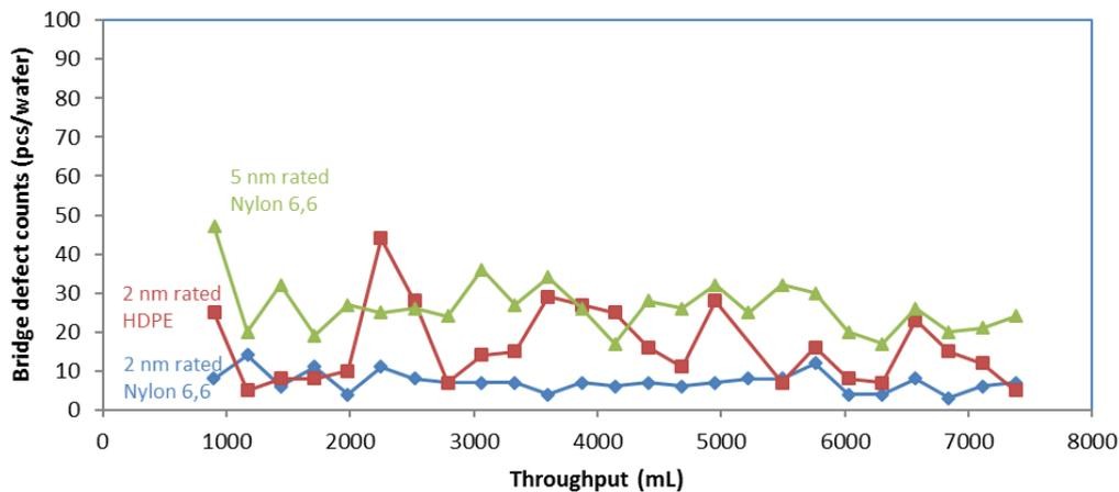
Figure 7. Bridge defect counts at 40 nm L/S pattern vs. throughput of POU filtration after replacing the pre-wet solvent to photoresist. Test fluid was TOK positive tone ArF immersion resist. Test filter format is Pall PhotoKleen EZD-3XL. Defect review was conducted using Applied Materials SEMVision G5.
