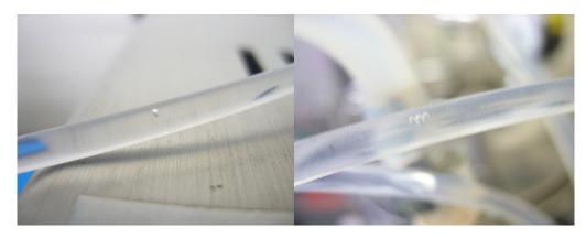
Figure 3. Visible bubbles found in the effluent of 30 nm HDPE filter.
